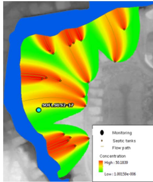
Figure 4-8. Simulated flow paths and plumes by the calibrated ArcNLET model in Martin County around well SOFLSUS2-17 (highlight in figure). Surface water bodies are plotted in blue.
