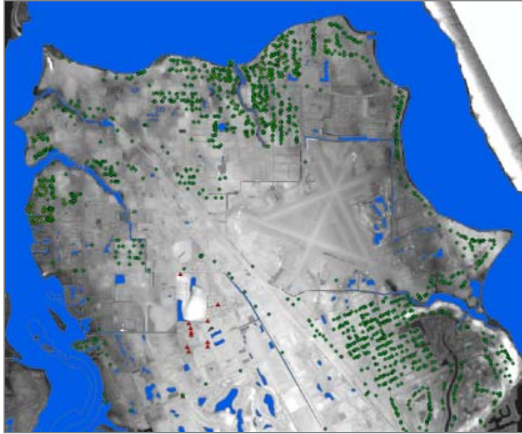
Figure 3-25. Locations of monitoring wells (red triangles) with nitrogen concentration data compiled from DBHYDRO. Septic systems in this area are denoted by green diamonds.
