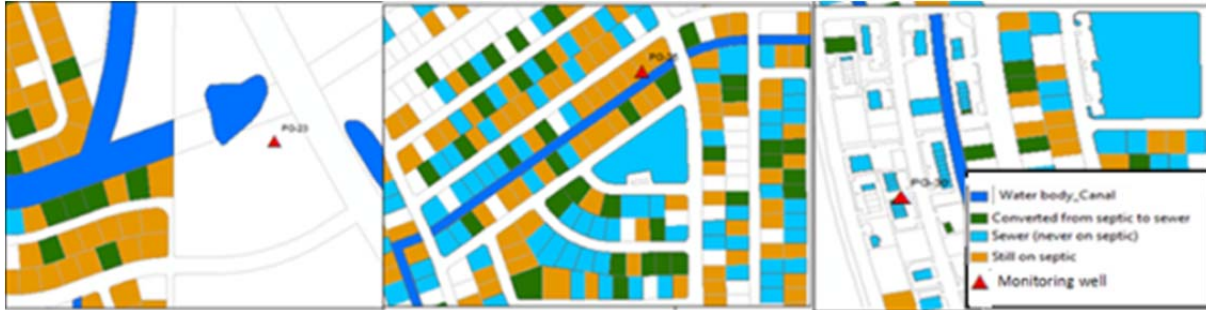
Figure 3-23. Locations of USGS monitoring wells (left: PG-23, middle: PG-25, right: PG-30) and septic systems surrounding the wells.
