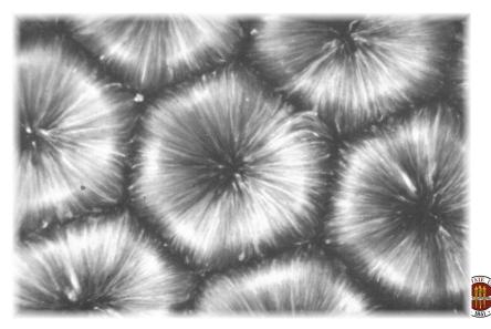
As water boils in a shallow, the hot water on the bottom of the pan rises to the cooler surface.
