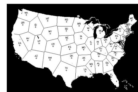
The Centroidal Voronoi diagram helps us to simulate, model, and sometimes to understand cell structures in which the generator tends to be in the center, or to move there:
